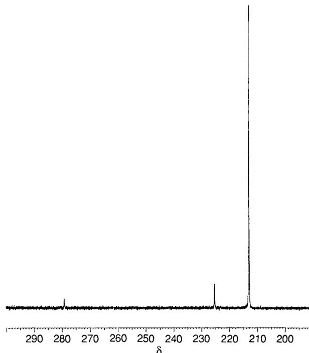
**Fig. 2** <sup>13</sup>C NMR spectrum of **4** in the CO region. (CD<sub>2</sub>Cl<sub>2</sub>, -30 °C). δ 279.1 (s, 1C, COMe), 225.2 (s, 2C, CO *cis* to the acyl group) and 213.0 (s, 1C, \*CO, *trans* to the acyl group).
